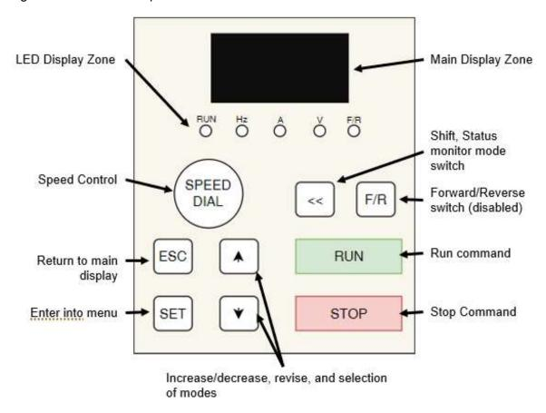
The main display of the Inverter will show information depending on what LEDs are lit in the LED display zone. Pressing the Shift << key will cycle between the different displays outlined below.
